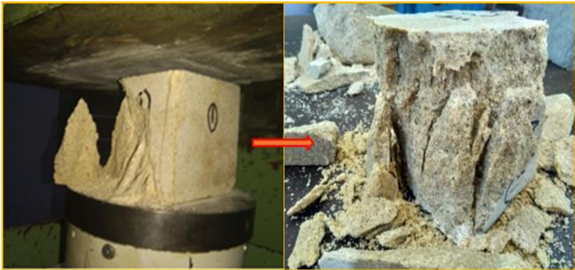
Figure 5.4. Failure of a coral stone cube under compression
