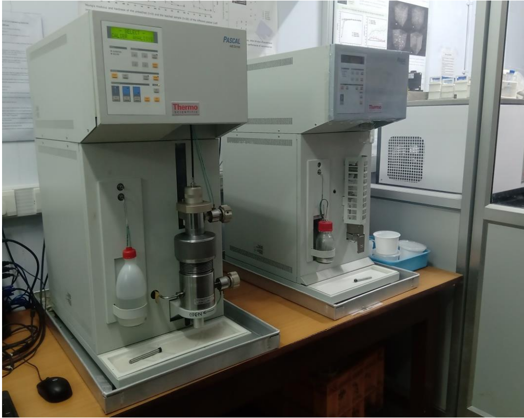
Figure 3.10. Thermo Scientific Mercury Intrusion Porosimeter
