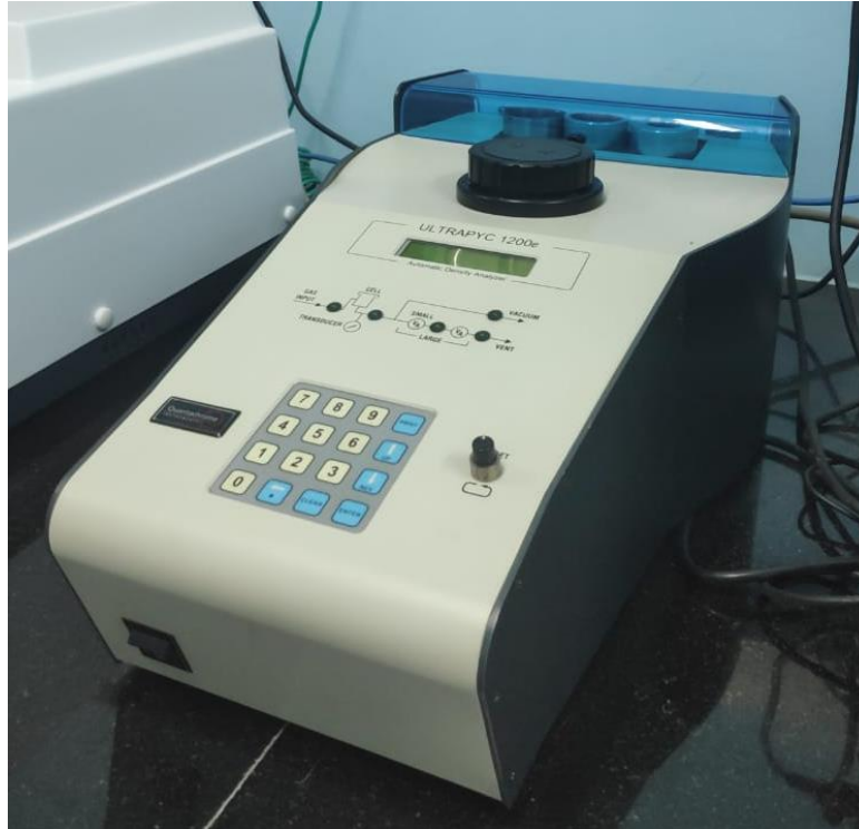
Figure 3.3. Helium gas pycnometer
