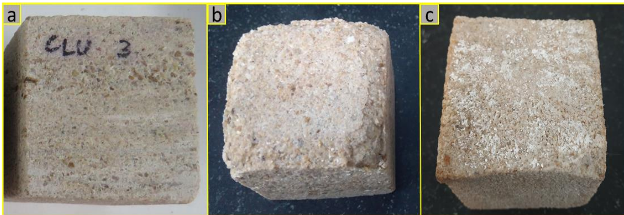
Figure 5.22. Coral stone specimens a) before subjecting to artificial weathering cycles b) after subjecting to \text{Na}_2\text{SO}_4 exposure c) after subjecting to \text{NaCl} exposure
