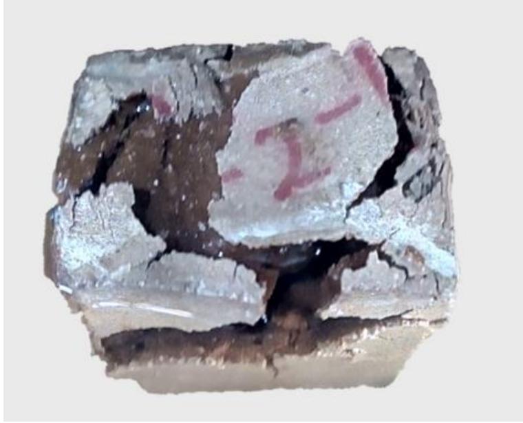
(a) Sudden rupture of C2 treated with SC coating at 15 cycles
