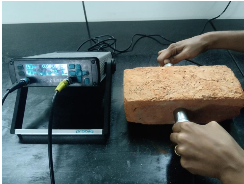
Figure 3.5. Illustration of UPV test on a brick sample
