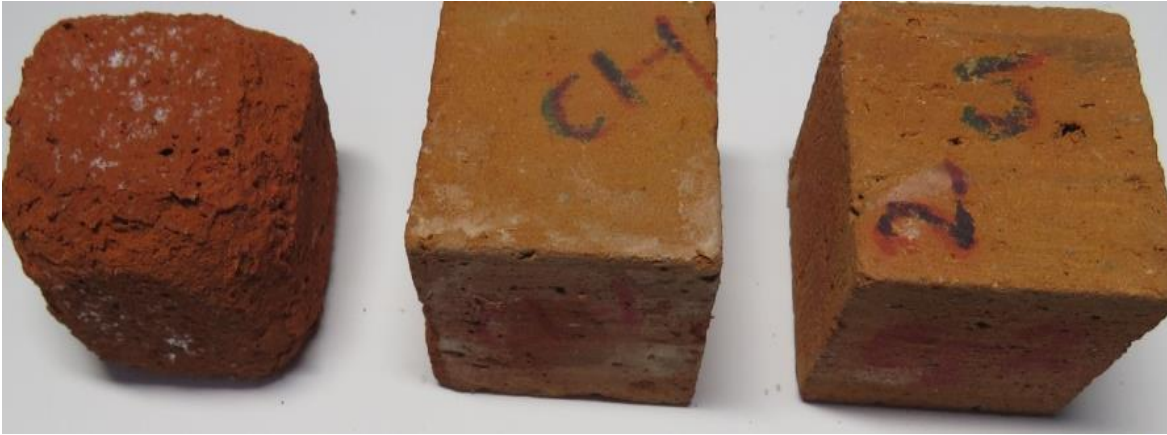
Figure 6.9. Damage state of specimens C1, C1-SC and C1-AS respectively after 20 weathering cycles
