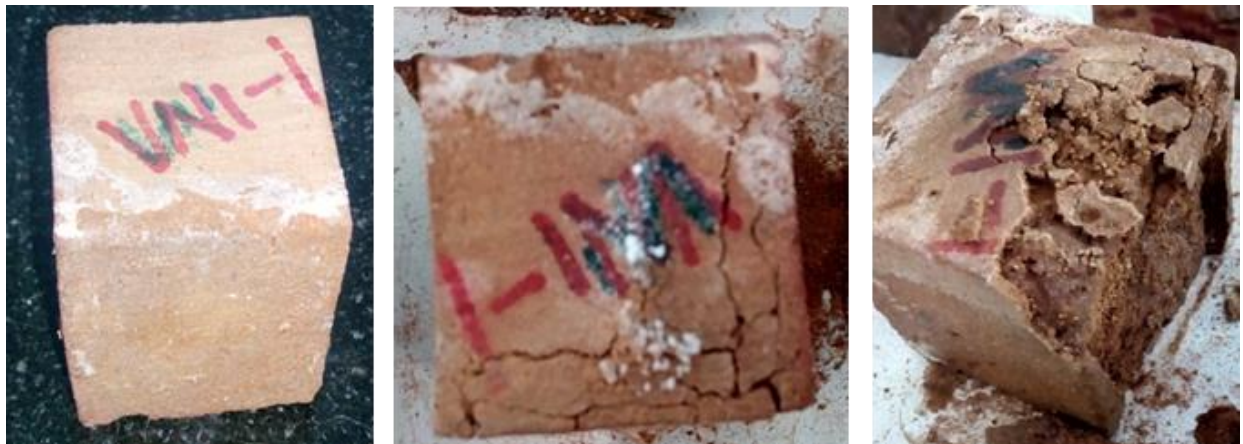
Figure 6.13. Sudden rupture of VN- specimen after 7th, 8th and 9th cycle respectively
