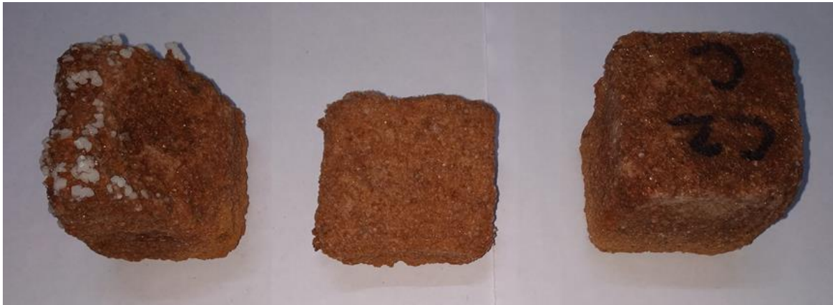
Figure 6.10. Damage state of specimens C2, C2-SC and C2-AS respectively after 20 weathering cycles
