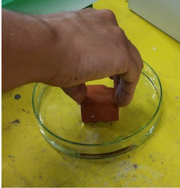
Figure 6.5. Illustration of cut specimen wetting with water to find penetration depth
