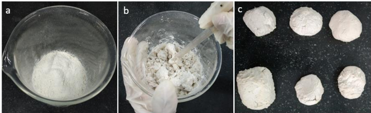
Figure 3.16. Steps followed in the process of poulticing (a) cellulose powder in the dry form (b) mixing of cellulose powder with water to prepare the poultice (c) samples covered with the cellulose poultice left for drying
